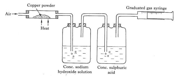
The above apparatus was set up to prepare nitrogen from the air. A slow stream of air was passed over the hot copper powder and nitrogen collected in the gas syringe.
